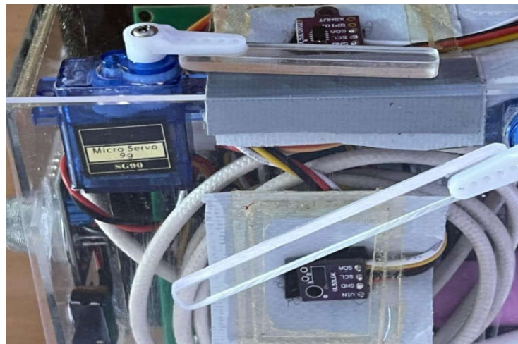
Fig. 10 Self-driven wiper mechanism for LiDAR lens cleaning.
