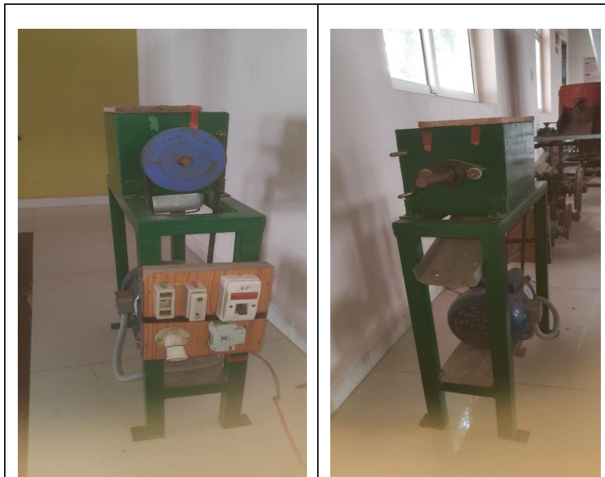
Figure 1: Sectional Views of Single-Shaft Shredder Machine
