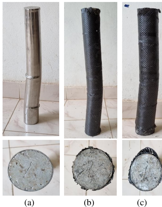
Fig. 4. Failure modes of LWCFST columns: (a) unconfined column, (b) confined with 1 layer of CFRP, and (c) confined with 2 layers of CFRP
