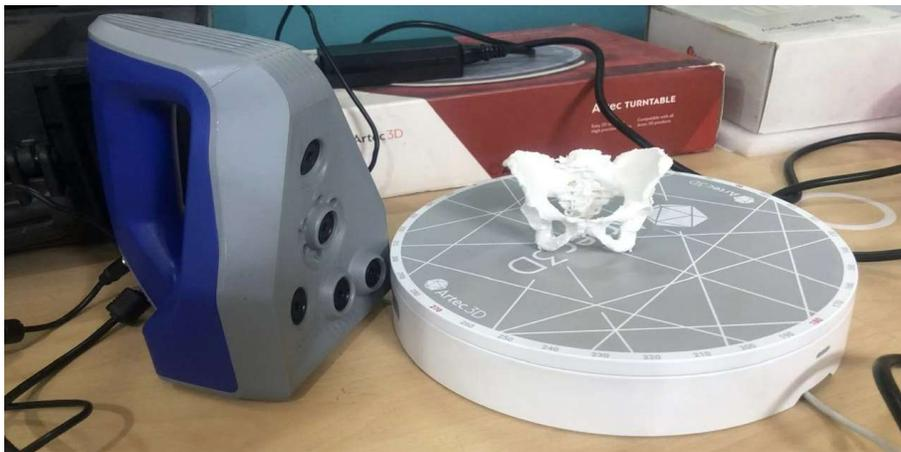
Fig 10: Artec Space Spider and Rotating table
