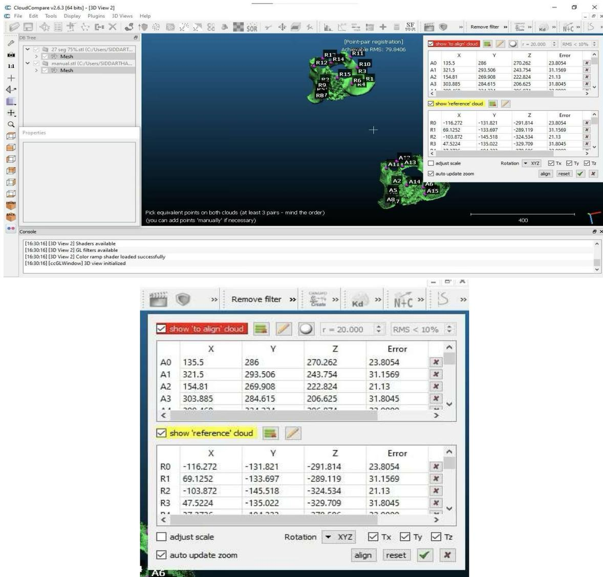
Fig 14: Point cloud alignment and mesh distance analysis using CloudCompare.
