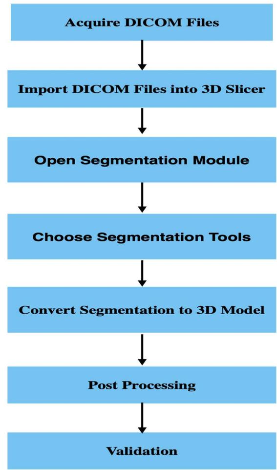
Fig 2: Process flowchart for manual segmentation
