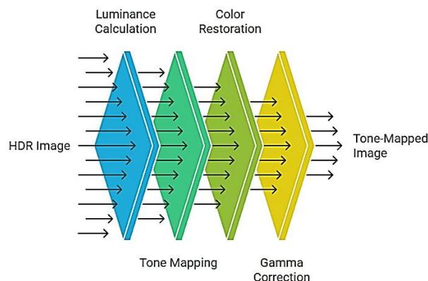
**Fig. 1.** Workflow diagram of tone mapping algorithm
