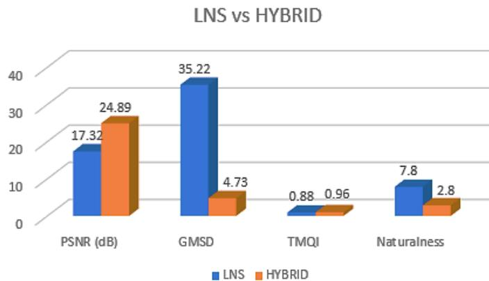
Fig 6.3: Graph showing comparison between LNS & HYBRID Model (Avg. values)
