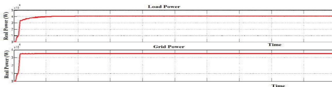
Fig.7.Power Outputs of Grid and Load during Daytime
