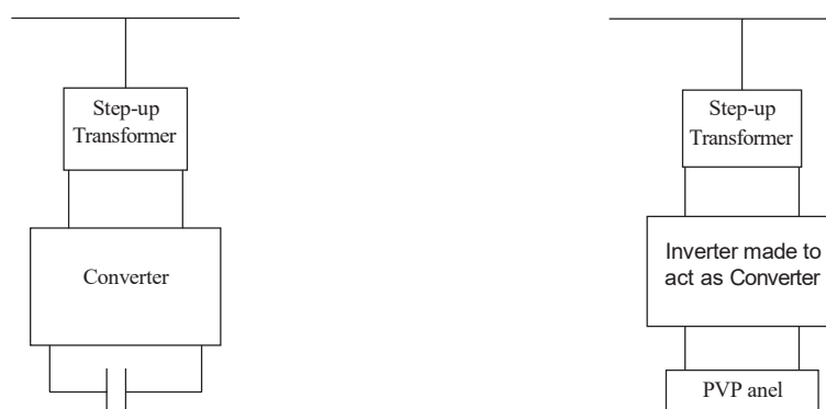
Fig.3. Conventional STATCOM vs. PV based Basic STATCOM Configuration
