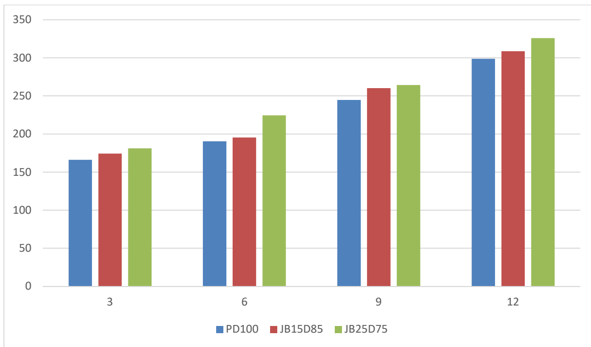
Fig.4.8: Load Vs Exhaust gas temperature
